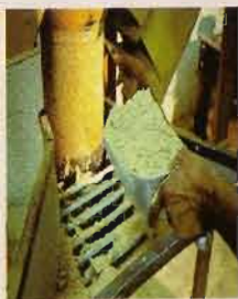
◀ A fishfood ingredient being introduced into a reduction mill to reduce the particle size to a coarse powder.
