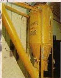
▲ The coarse powder is delivered to a micropulverizer further reducing the ingredients to micron size.
