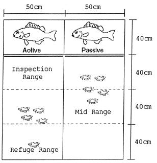
*Fig. 1:* Diagrammatic view of the experimental tank used in expt 1 showing the divisions into the three ranges (inspection, mid and refuge). A clear Perspex divide and an opaque division, which could be drawn up by a pulley system to reveal the predators to the prey, separated the predators from the rainbowfish
